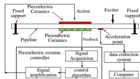
Figure 1 The principle diagram of the test
