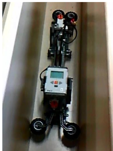
Figure 7 Robot Earthworm: A robot moves itself according to the expansions and contractions in different dimensions of the body.
