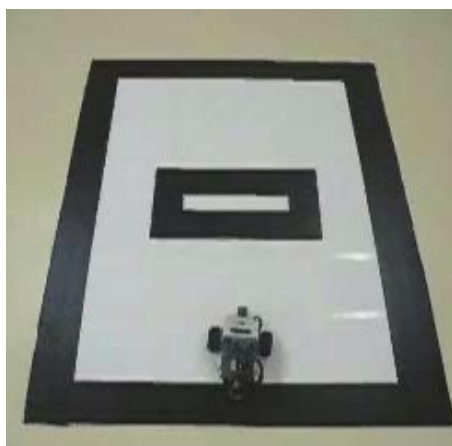
Figure 10 Robot Beetle: Robot goes up side avoiding to crash to the black lines in the center of the square according to the optimization result of genetic algorithm. Download the video (591KB):
