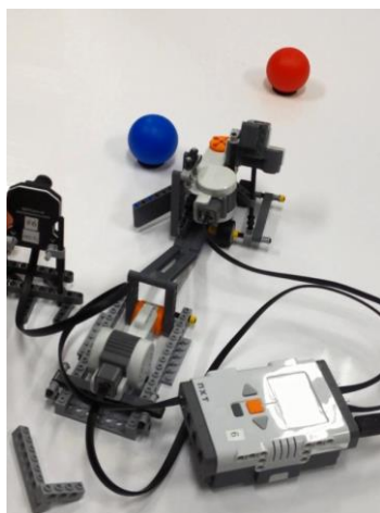
Figure 6 Robot Batter: Robot calculates the position of the red ball by the camera, and changes the angle of an arm which hits the blue ball to the red one. Download the video 21.7MB: http://www.nn.csse.yamaguchi-u.ac.jp/video/batting.wmv
