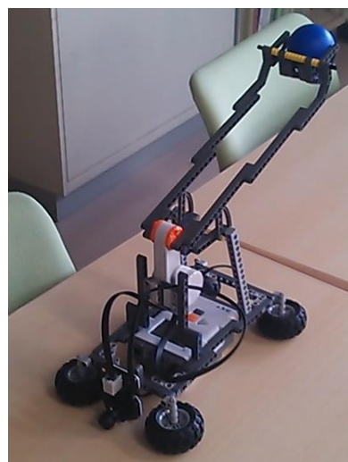
Figure 8 Robot Throwing: A robot throws a blue ball to attack a red ball in front of it by calculating the variable distance using images captured by a camera. Download the video (10.5MB):
