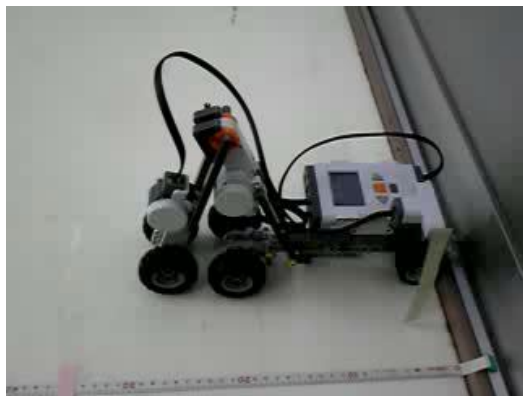
Figure 9 Robot Inchworm: Robot moves to a destination by the movement of expansion and contraction of the arm according to the learning result of reinforcement learning. Download the video (1.52MB):
