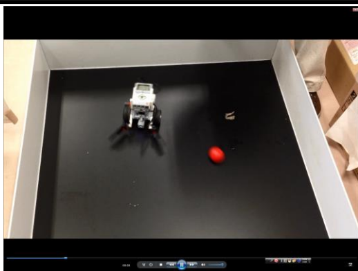
Figure 13 Ball Playing Robot: A robot can recognize the color of the ball in front of it and throw it quickly with different direction according to the color of the ball. Download the video (15.3MB): http://www.nn.csse.yamaguchi-u.ac.jp/video/hirameki_geshi.wmv
