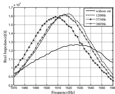
Figure 5 Impedance Variation Corresponding to Concentration of Mixture
