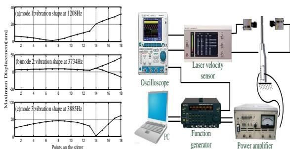
Figure 2 Experiment Setup of Vibration Mode Test
