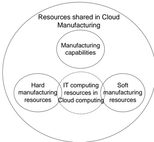
Fig. 2 Manufacturing Resource Sharing Model of Cloud Manufacturing [2]
