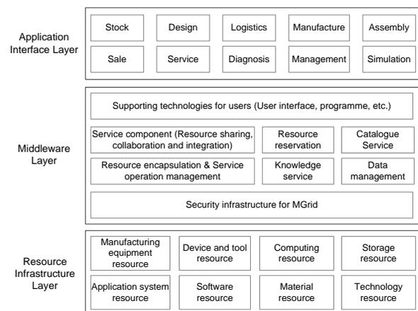
Fig. 1 Manufacturing Resource Sharing Model of MGrid
