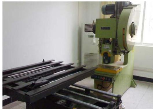
(b) Punching machine used in functional tests
