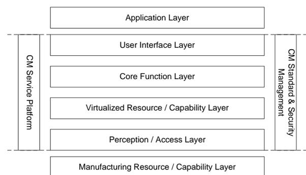
Fig. 4 Layered System Framework of Cloud Manufacturing
