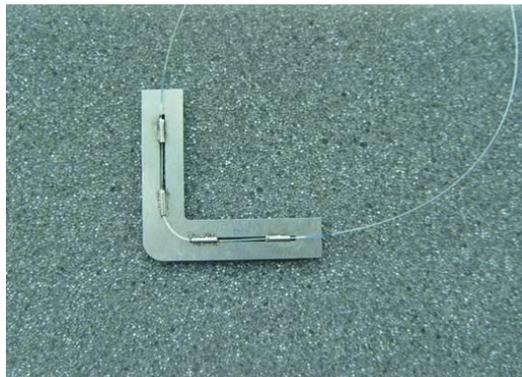
(b) The developed fiber optic sensors
