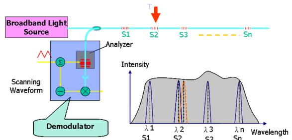
Fig. 10 Distributed Monitoring Method using FBG Sensors
