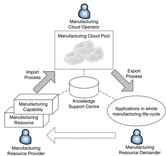
Fig. 6 Technological System of Cloud Manufacturing [9]
